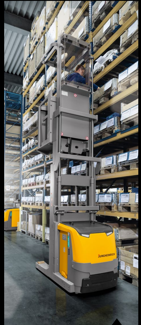
The EKS 110. Ideal for order picking up to the third rack level.
