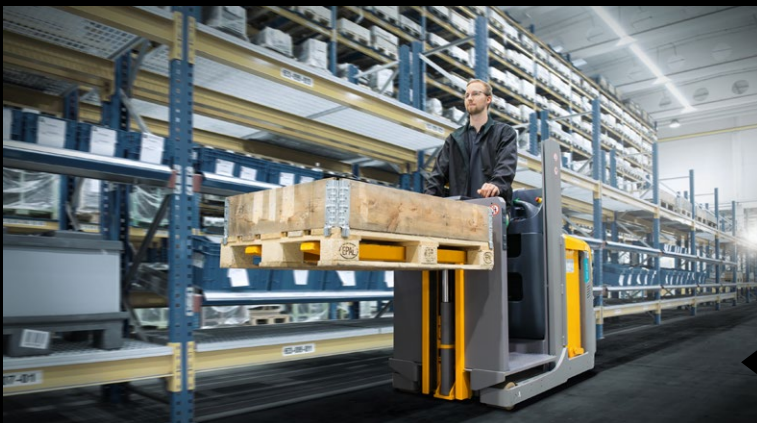
Energy recovery with regenerative braking. Standard from series 1.
